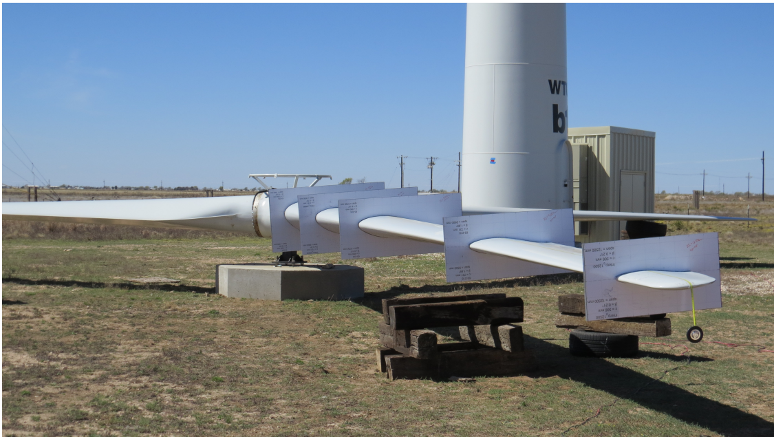
Figure 2.2. Foam templates fit onto V27 WTGb1 blade.
